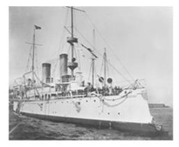
Length: 344 feet Beam: 53 feet Displacement: 5,870 tons Crew: 33 Officers, 396 enlisted men Top Speed: 22 knots (25mph) Coal Consumption at Top Speed: 633 lbs./minute
